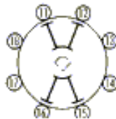
Fig. 16 Two pole per section, double break switching assembly.
