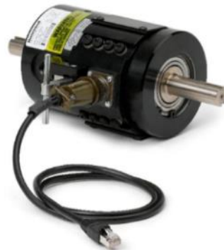
Fig.50 Rotary slip ring torque sensors can be used to measure startup, running, and stall torque levels
